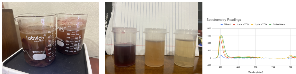
Figure 1: A Mycoremediation Experiment. The figures, left to right, show the experiment testbed, color change from start (leftmost), single cycle experiment (middle) and 2 cycle experiment (right). The final figure shows the spectrometry graph, indicating that while both experiments show value, the second approach gets much closer to distilled water
