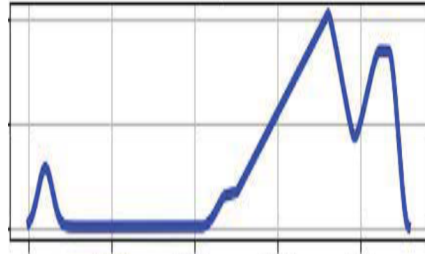
Figure 3: An example laser pulse shape used in ICF experiments. The shape is controlled by 5 parameters. The parameters are adjusted during an optimization campaign to maximize energy yield.
