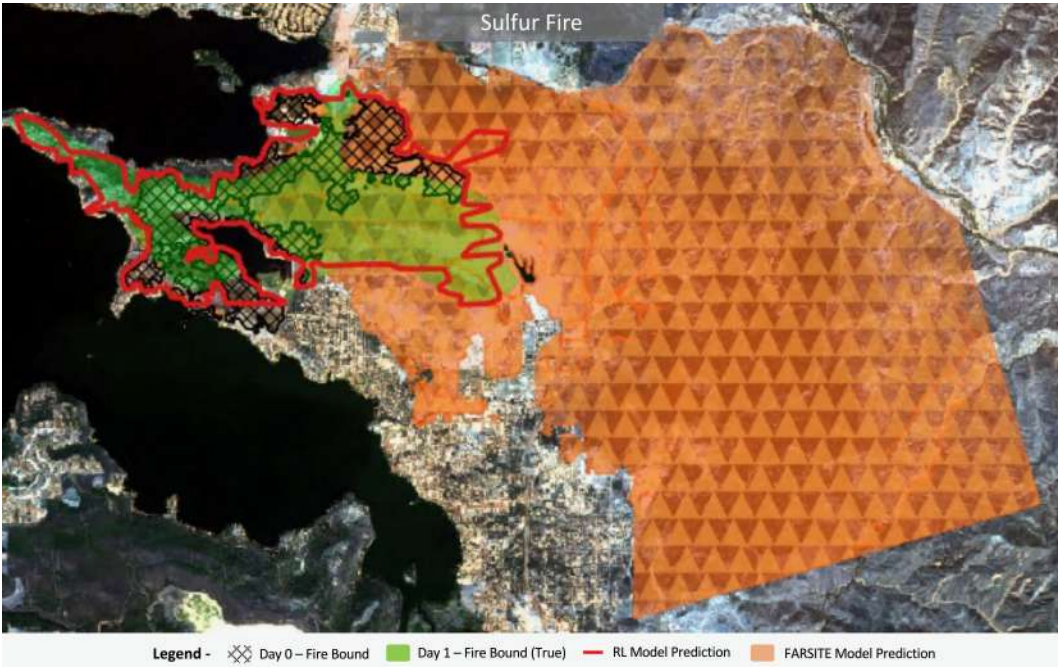
Figure 4: Imagery of site of Sulfur Fire via RapidEye program with RL and FARSITE predictions
