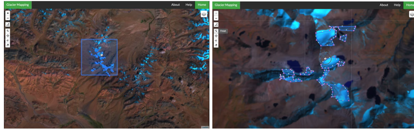
Figure 4: The image on the left shows the polygonized prediction for an area of interest. The image to the right shows the tool's functionality of allowing users to correct predictions.
