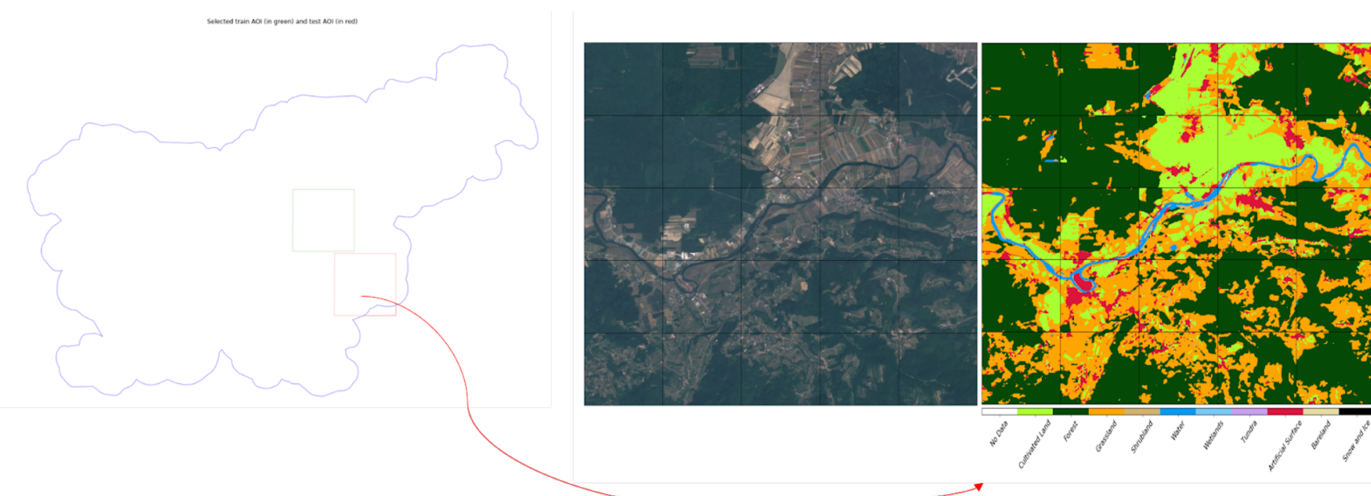
Figure 2. The pipeline fetches training data, Sentinel-2 optical imagery and labeled 10 classes LULC, for the AOI (in green) that covers 1296 km2 in Slovenia. A UNet using ResNet50 as the encoder was trained, and the model prediction was done over a new area (in red), and the LULC classification is shown on the right.
